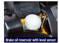
The enhanced brake oil reservoir, located in the upper left dash is equipped with an electronic level sensor and easily visible through the monitor.
