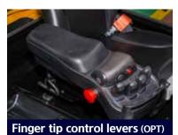
Ergonomically designed fingertip control levers for improved operator comfort and productivity. The armrest can be adjusted for operator comfort.
