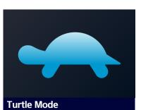
When selecting the turtle mode while working in narrow and congested workplace, the travel speed is reduced at a preset speed.
