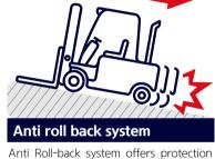
Anti Roll-back system offers protection against the machine rolling back on a ramp in combination with exceptional ramp start capabilities.
